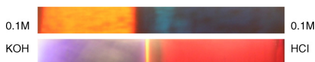
Fig. 10. Position of the acid–base boundary visualized by congo red and thymol blue (the upper and bottom image, respectively) when no external electric field is applied to the system. The images have been converted to the greyscale with enhanced contrast for printed edition, to see original colours please cf. the on-line edition.
