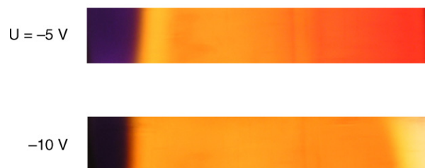
Fig. 11. Experimental results for negative external potential difference (i.e., the diode in the open mode) for thymol blue in Agar gel. For potential difference -5 V the left dark field marks the area of pH above 9, the lighter central part (yellow in reality) denotes the area with pH value between 9 and 2 approximately, the dark right border of the image (red in reality) denotes pH below 2. When the external potential difference U has been set to -10 V, the red-coloured area disappeared. The images have been converted to the greyscale with enhanced contrast for printed edition, to see original colours please cf. the on-line edition.
